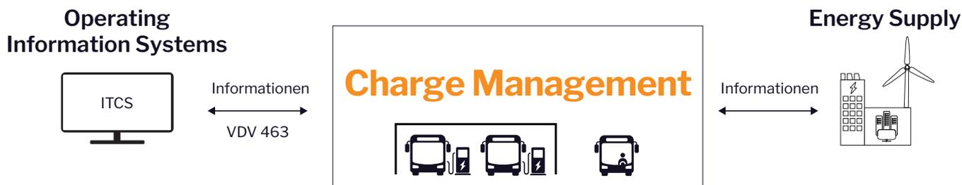
A complex data exchange is required to manage e-bus charging processes.
