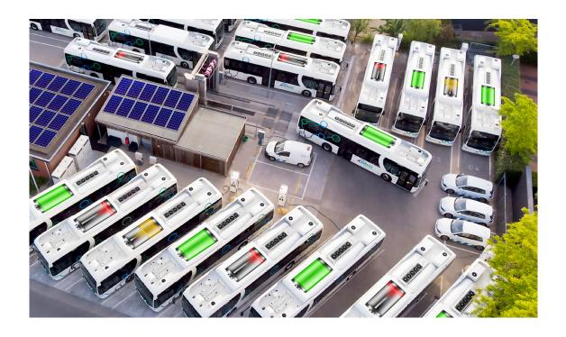
With more electric buses in the fleet, there is an increased need for well-coordinated charging. After all, a large number of vehicles will require a significant amount of power within a relatively short time frame. MOBILEcharge ensures parallel, controlled, and automated charging processes at the depot by connecting charging points, the electricity supply, and operational information systems.
