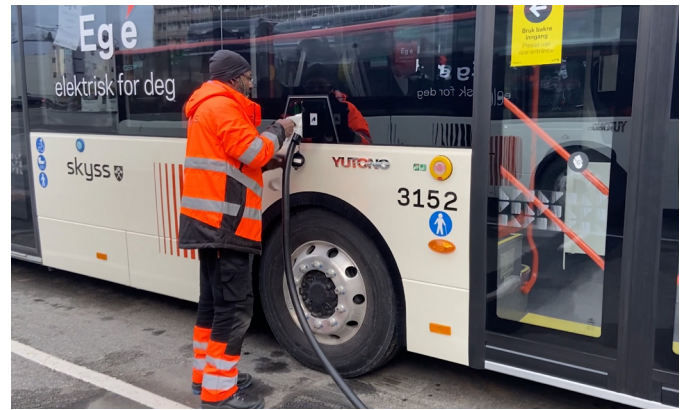
Electric bus is preconditioned while plugged in.
