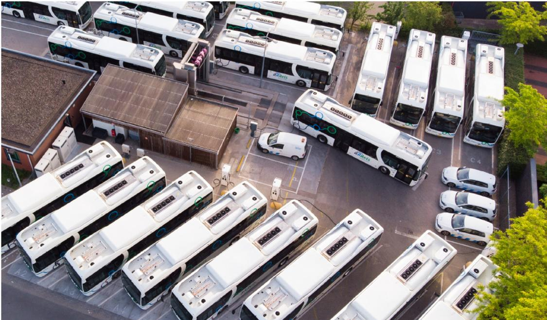
With more electric buses in the fleet, there is an increased need for well-coordinated charging. After all, a large number of vehicles will require a significant amount of power within a relatively short time frame. MOBILEcharge ensures parallel, controlled, and automated charging processes at the depot by connecting charging points, the electricity supply, and operational information systems.
